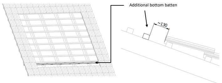
**Note:** The length of additional battens should be specified according to the number of solar collector panels in the array.
