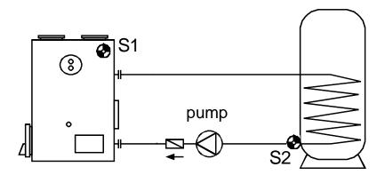
The pump runs when sensor **S1** is greater than the *min* threshold and sensor **S1** is higher than sensor **S2** by the *diff* differential.
