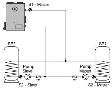
• 2-pump mode: as can be seen in the schematic diagram, a pump is connected to both master and slave. The master pump has absolute priority, hence the slave pump can only be switched on if the master pump is switched off (dependent on the starting conditions). 2-pump mode is activated if the terminals of the boiler sensor at the slave remain disconnected (= lead break).
