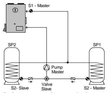
Pump-valve mode: the common pump is connected to the master controller, the slave
