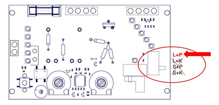
The selection occurs by means of a slide switch on the right border of the board. There is no access possible to the slide switch from outside. Four positions are available.
