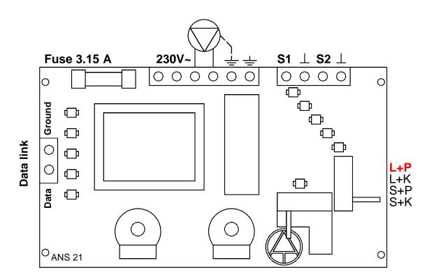
When using the master-slave function, the data link must be connected **in-phase** to both units (data to data, ground to ground).
