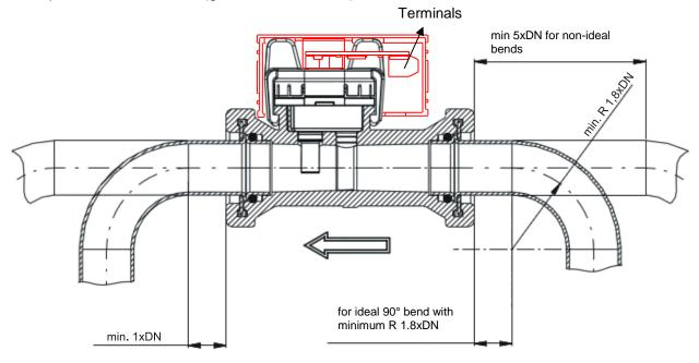
The flow direction must be observed without fail (indicated on the sensor by an arrow). The fitting position can be freely selected.
