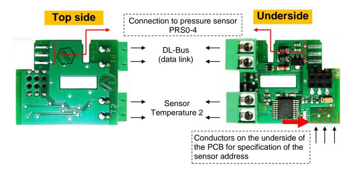
The polarity of the connections ("earth") is interchangeable, hence is unimportant.
