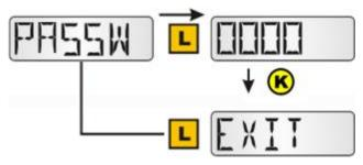
The purpose of this password is to block access to the CONFIG and VALUES menus. For access, enter the password set here. If 0000 is entered, no password is required. While the password is shown, long clicks can be used to go through the individual character places (active place flashes) and a short click increases a place by 1. A long click while the last place is
