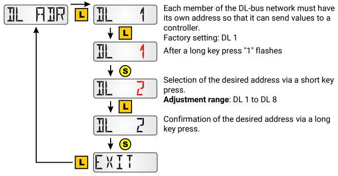
Among those controllers that have no bidirectional data link (e.g. HZR65), i.e. those for which the **RAS+DL** can only be used as a **remote display**, this menu option is still displayed but has no effective function and must therefore not be observed.
