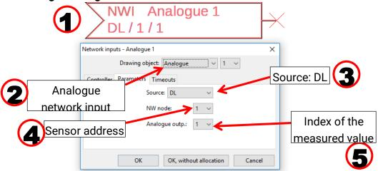
A still unused network input variable must be selected for each new value. The values of the indices 1 and 5 displayed at the network input do not correspond to the temperatures and are only correctly displayed in the controller in the measured values overview and in the functions.
