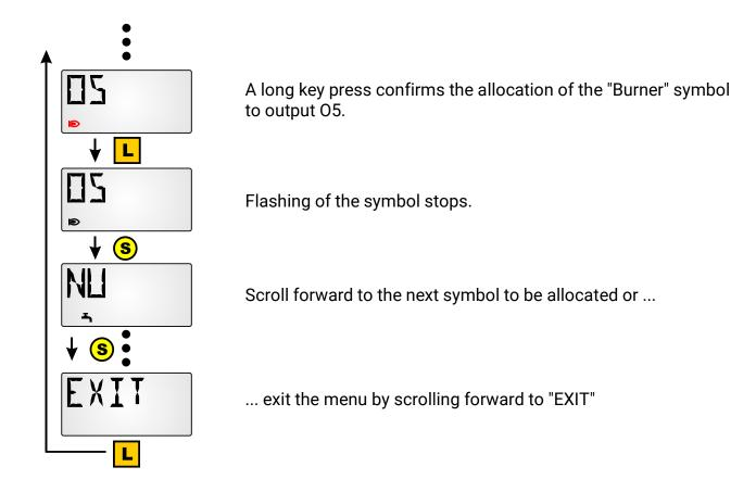
If the symbol is allocated to an **Output** or a **Digital CAN network input** (UVR1611), then it is shown in each display view for as long as the output or the digital network input is set to "ON".
