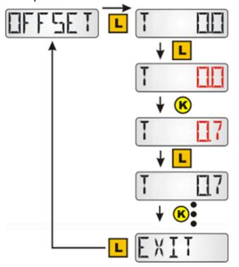
Entry T 0.0 = no offset value selected, therefore no sensor correction Factory setting: T 0.0
